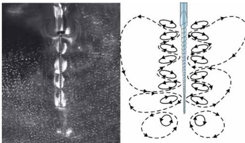
Fig. 1: Acoustic streaming around a file in free water (left) and a schematic drawing (right)
