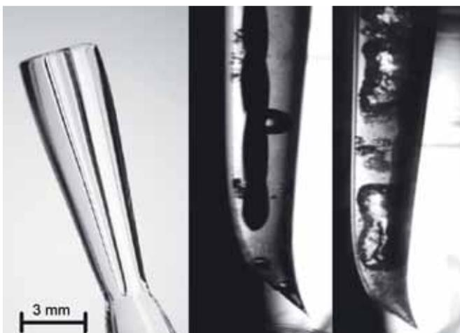
**Fig. 2:** Left: Glass root canal model allowing optical access to the vibrating file for high-speed visualization of ultrasonic irrigation. Middle: File in operation captured at microseconds time scale displaying both transient and inertial cavitation phenomena and, in addition, local streaming patterns (only visible in video mode), right: a high-speed recording of a noncutting K-file is shown, displaying vigorous microstreaming and collapsing cavitation bubbles
