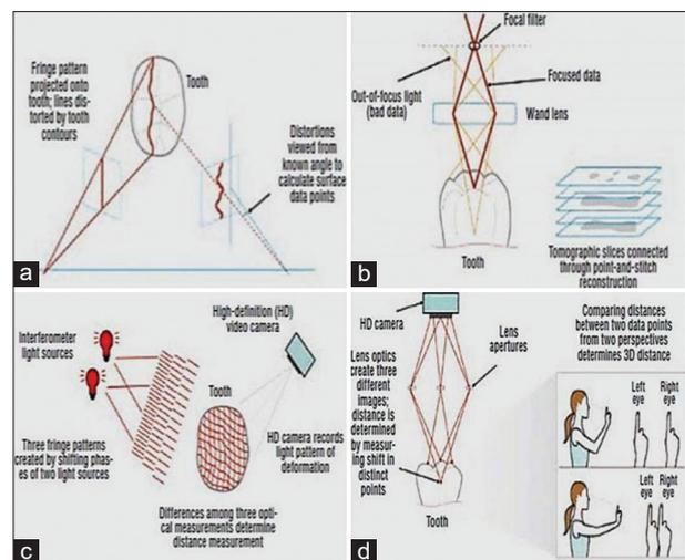
Figure 5: (a) Triangulation technique (b) paralleling confocal technique (c) accordion fringe interferometry (d) active wavelength sampling
